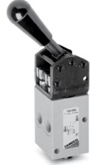
The Series 3 manual valves (G1/8, 3/2 and 5/2-way) and the Series 4 manual valves (G1/4, 3/2, 5/2 and 5/3-way) are available with devices designed to satisfy different needs. The 3/2-way valves Series 3 and 4) are normally closed when 1 is the inlet; they can also be normally open when 3 is the inlet.
