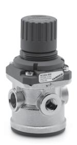
The Series N pressure regulator is available with G1/4 and G1/8 ports. Its design incorporates a self relieving diaphragm so as to allow decremental adjustments.
