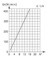
Flow Qn (Nl/min.) from  $2 \rightarrow 1$  with controller OPEN: 530 Flow Qn (Nl/min.) from  $2 \rightarrow 1$  with controller CLOSED: 160 Qn is determined with a supply pressure of 6 bar and with  $\Delta P = 1$ bar at the outlet
