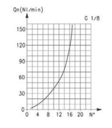
Flow Qn (Nl/min.) from  $2 \rightarrow 1$  with controller OPEN: 200 Flow Qn (Nl/min.) from  $2 \rightarrow 1$  with controller CLOSED: 70 Qn is determined with a supply pressure of 6 bar and with  $\Delta P = 1$ bar at the outlet
