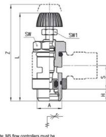
Note: M5 flow controllers must be used together with M6 adjustable fittings.
