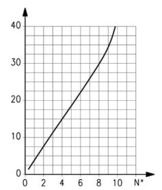
Flow Qn (Nl/min.) from 2  $\rightarrow$  1 with controller OPEN: 47 Flow Qn (Nl/min.) from 2  $\rightarrow$  1 with controller CLOSED: 33 Qn = supply pressure of 6 bar and with  $\Delta P$  = 1 bar at the outlet N° = number of screw turns.
