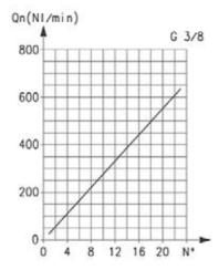
Flow Qn (NI/min.) from 2  $\rightarrow$  1 with controller OPEN: 710 Flow Qn (NI/min.) from 2  $\rightarrow$  1 with controller CLOSED: 410 Qn is determined with a supply pressure of 6 bar and with  $\Delta P$  = 1 bar at the outlet.
