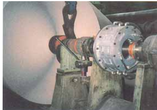
Conversion of Bruderhaus winder with CSM 221 Brake
