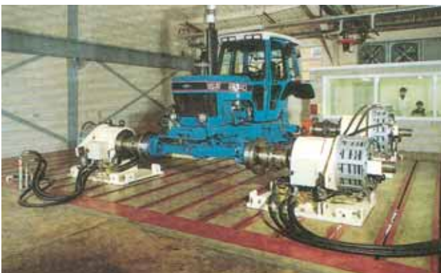
Plint & Partners Advanced Axle Dynamometer at Silsoe Research Institute, Bedford —CSM 224 Brakes on Front Wheels, CSM 130 Brake on Rear Wheels.
